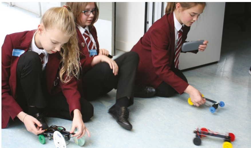
Solar-powered cars - students could change the gearing and wheel size to make them faster
